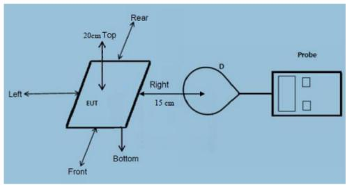
Remark: The EHP 200A probe antenna diameter is less than 11.5cm.
