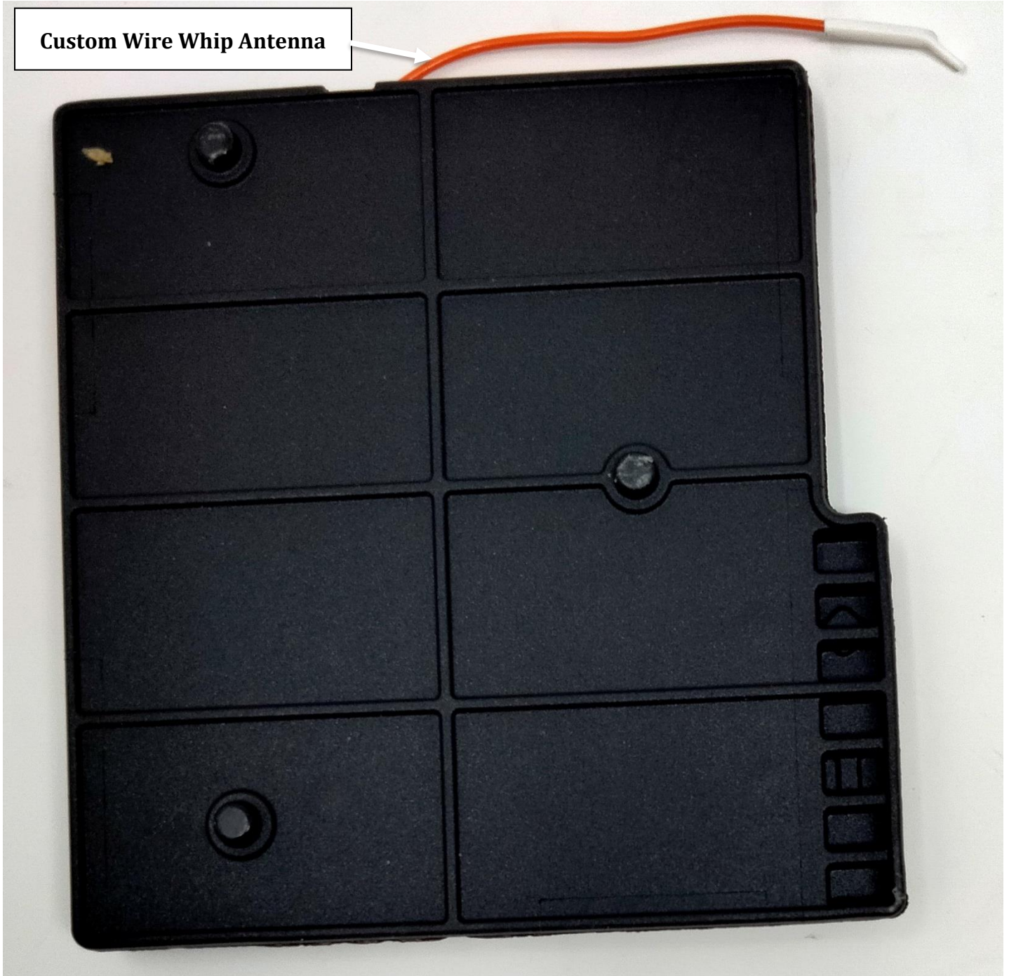
Bottom View of EA144 (In Molding)
