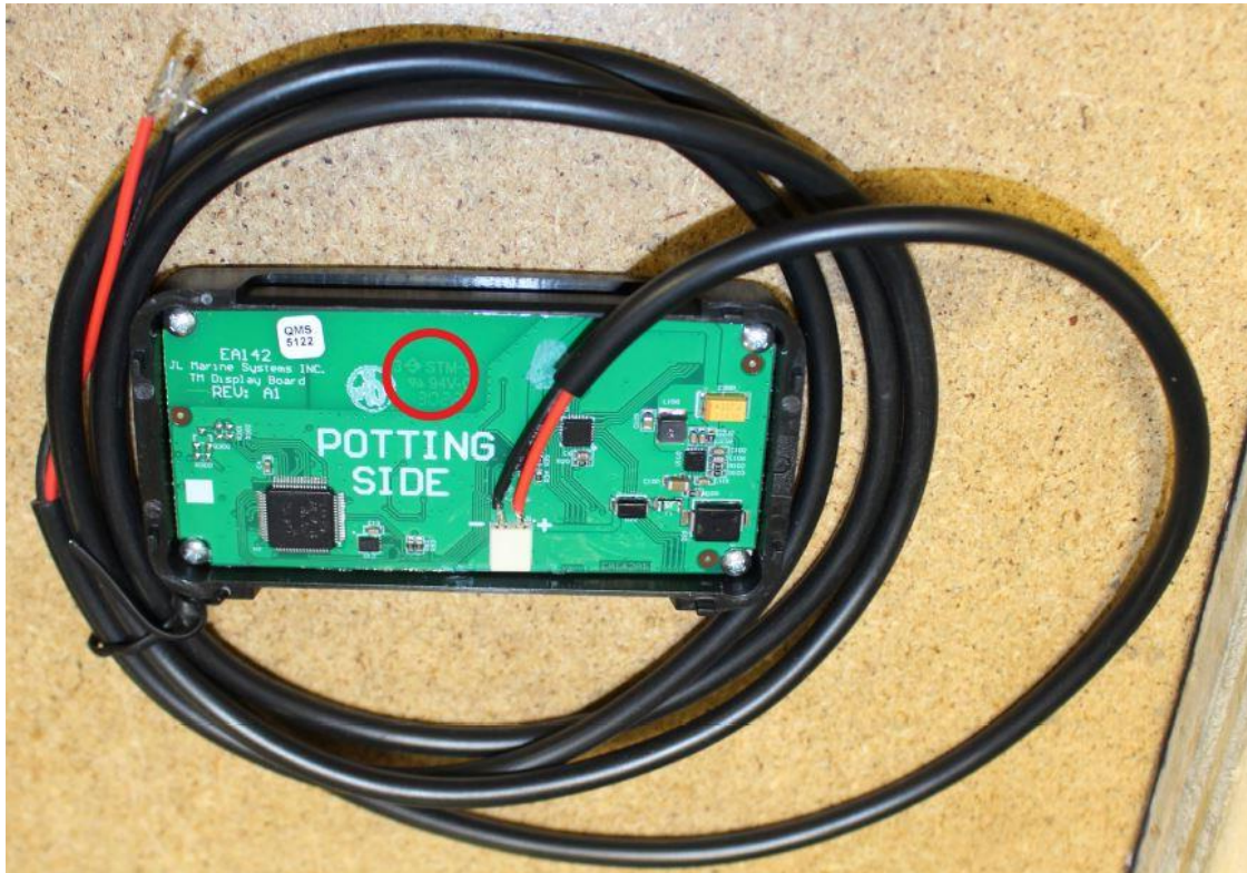
Bottom View of EA142 (In Unit Before Potting)
