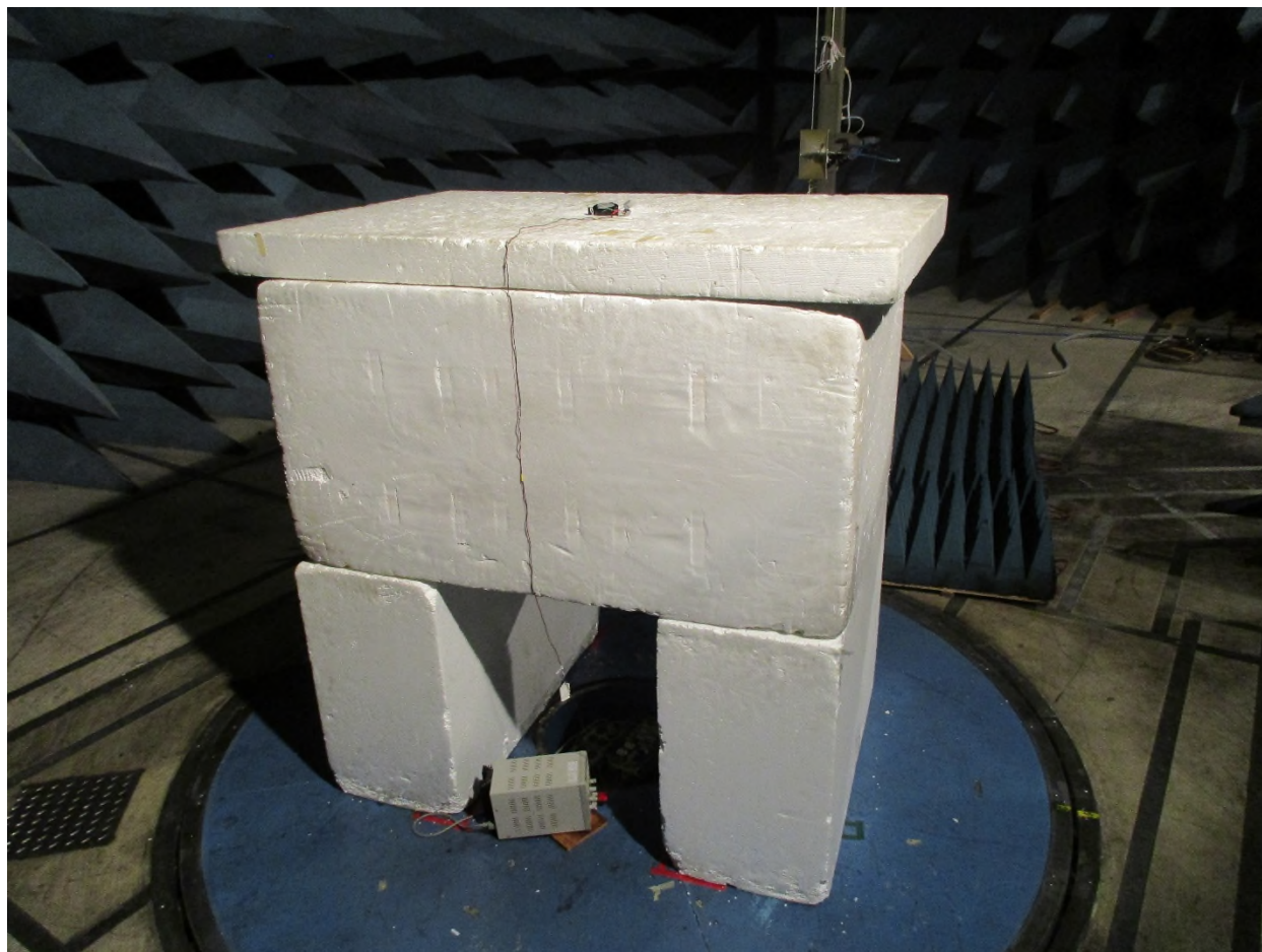
Figure 6: Radiated Emissions Setup above 1 GHz – Rear View
