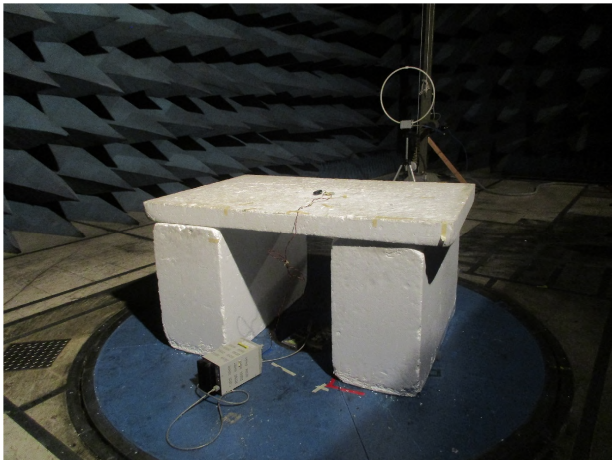
Figure 2: Radiated Emissions Setup 9 kHz to 30 MHz – Rear View
