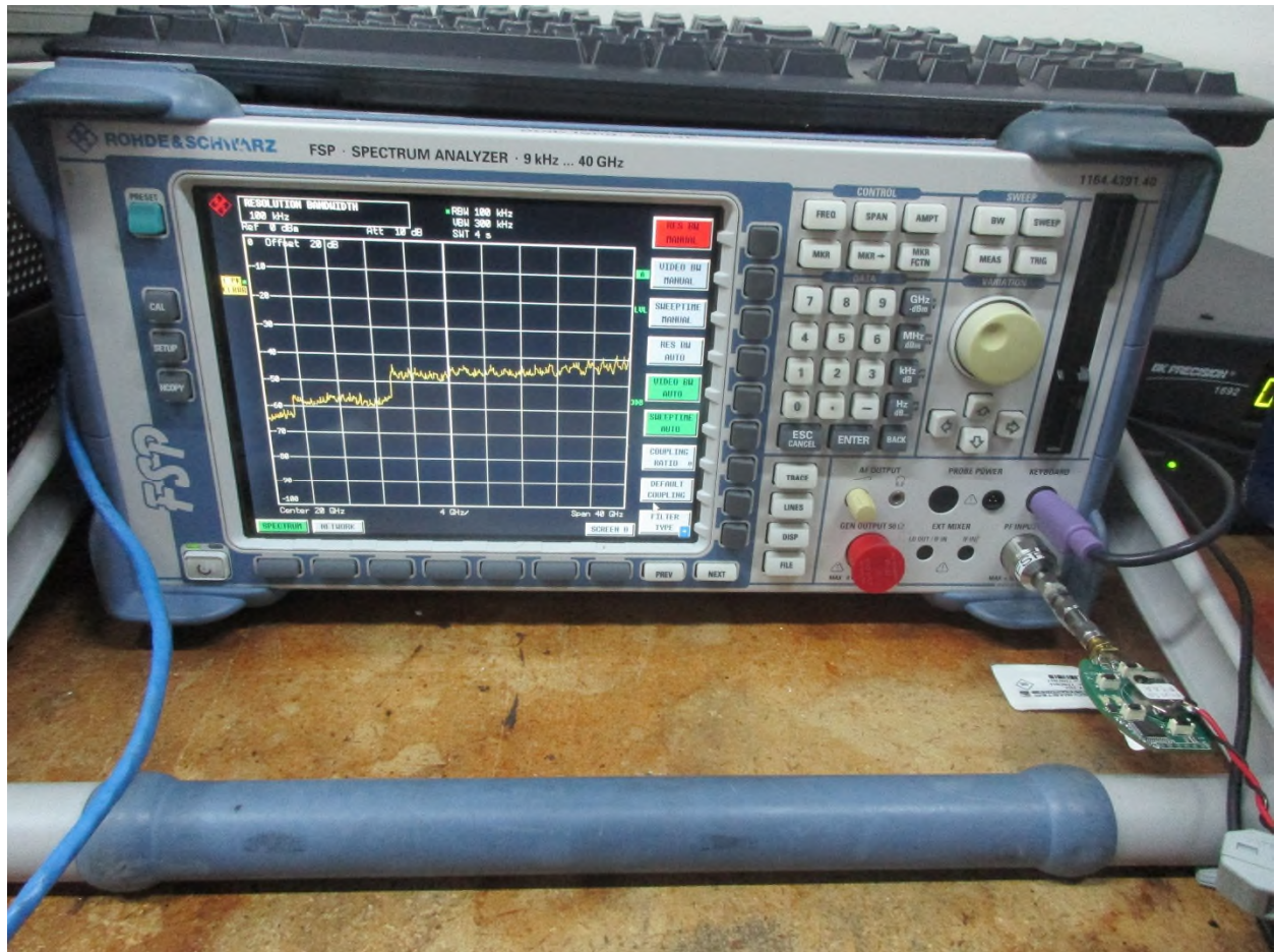
Figure 7: RF Conducted Measurements
