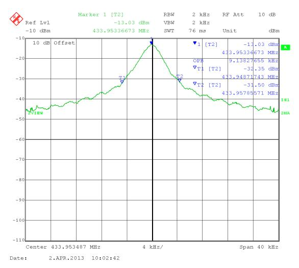
20 dB OCCUPIED BANDWIDTH = 9.1 kHz
