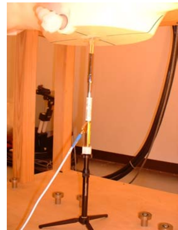
2450MHz System performance check setup
