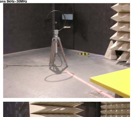
2 Photographs of Radiated Emissions Test Configuration
