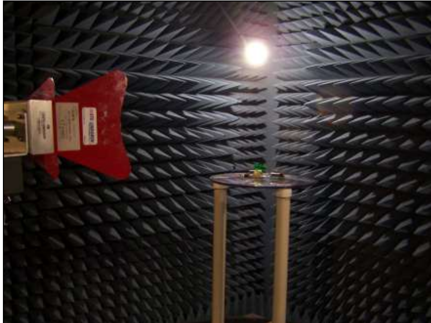
Photograph 3. Radiated Spurious Emissions, Test Setup, Above 1 GHz
