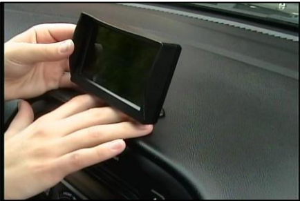
Adhere the monitor to the dash. 1
