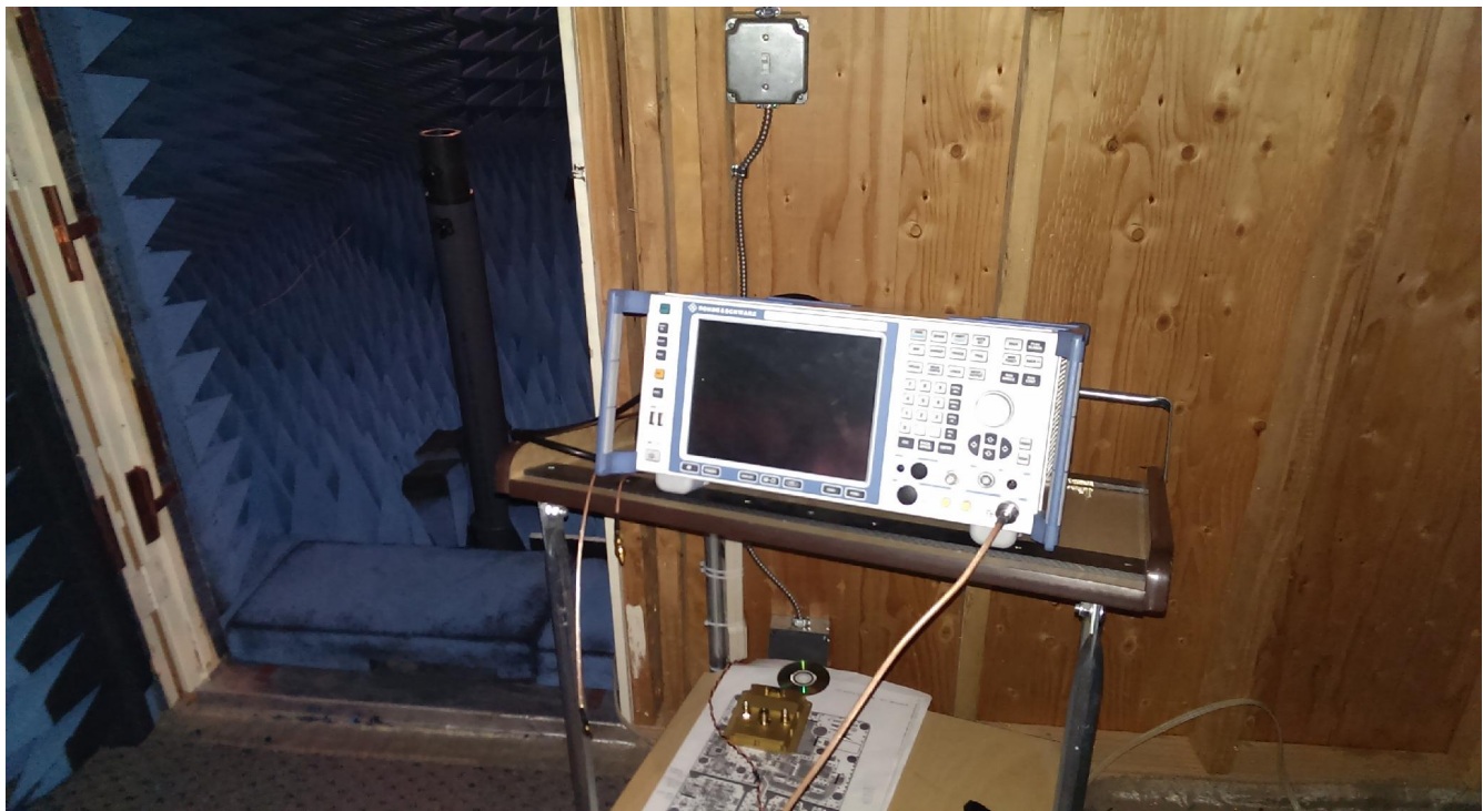
Illustration 86: Radiated Emissions Test Setup. Receiver Spectrum Analyzer is located outside of the anechoic chamber on the receiver Standard Gain Horn side.
