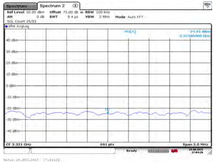
Illustration 32: Spectrum @ 2nd harmonic frequency
