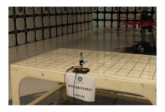
Radiated Emissions Test Setup (below 1GHz)
