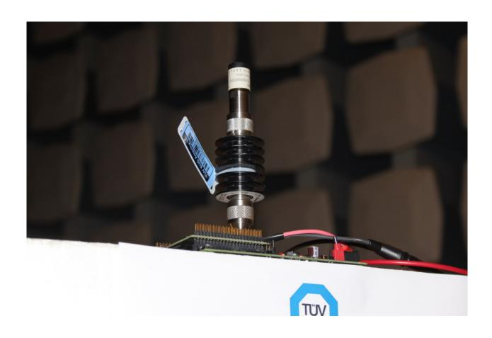
**Radiated Emissions Test Setup**
