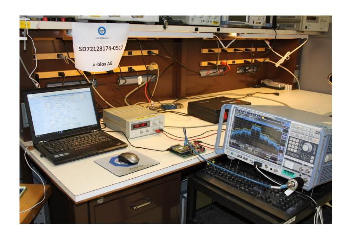
**Antenna Conducted Port Test Setup**
