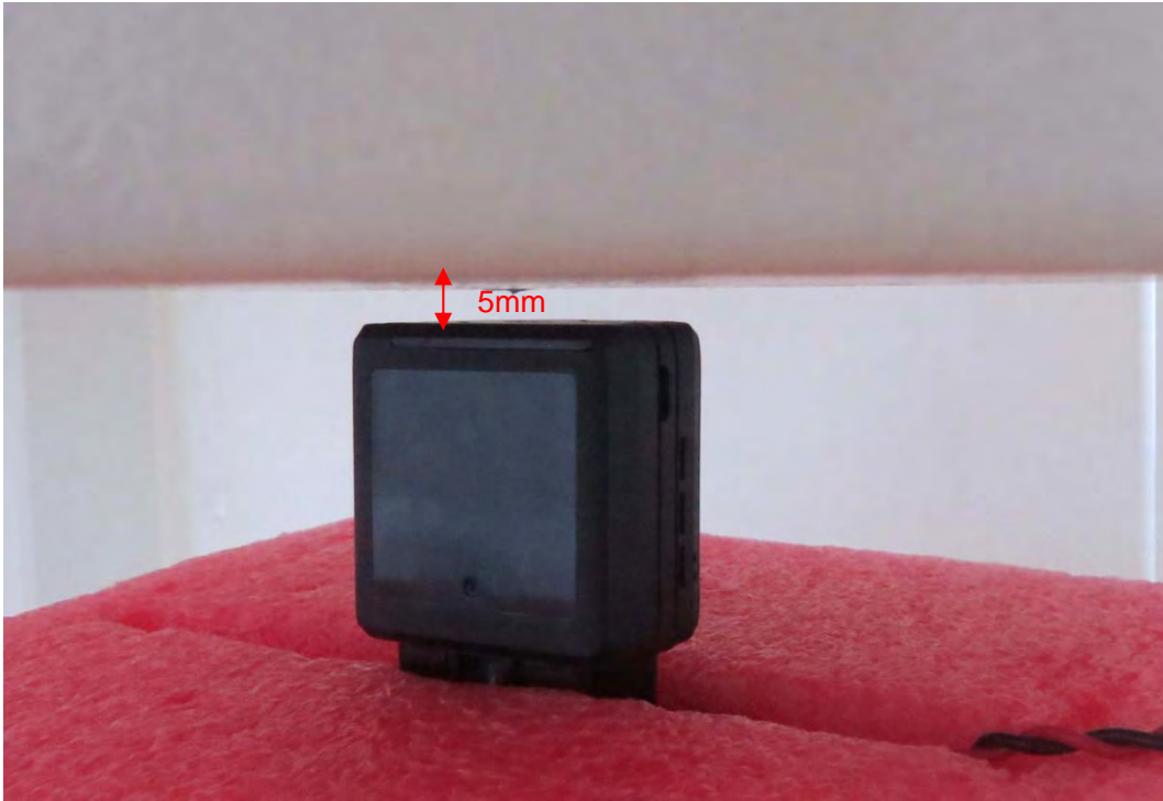
Picture 11: Top Edge, the distance from handset to the bottom of the Phantom is 5mm
