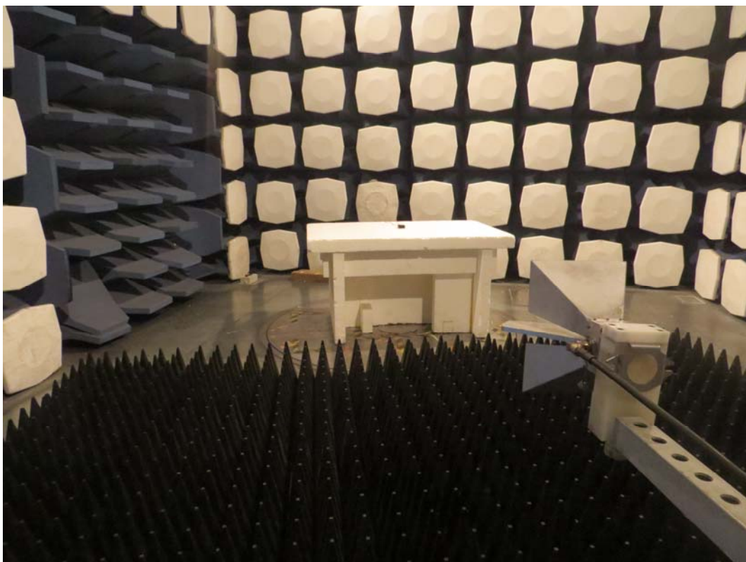
Picture 2: Radiated Spurious Emissions Test setup
