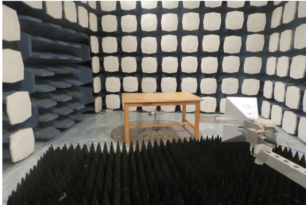
Picture 2 Radiated Emission Test Setup
