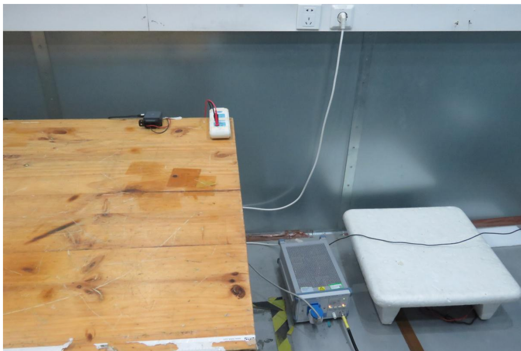
Picture 3 Conducted Emission Test Setup
