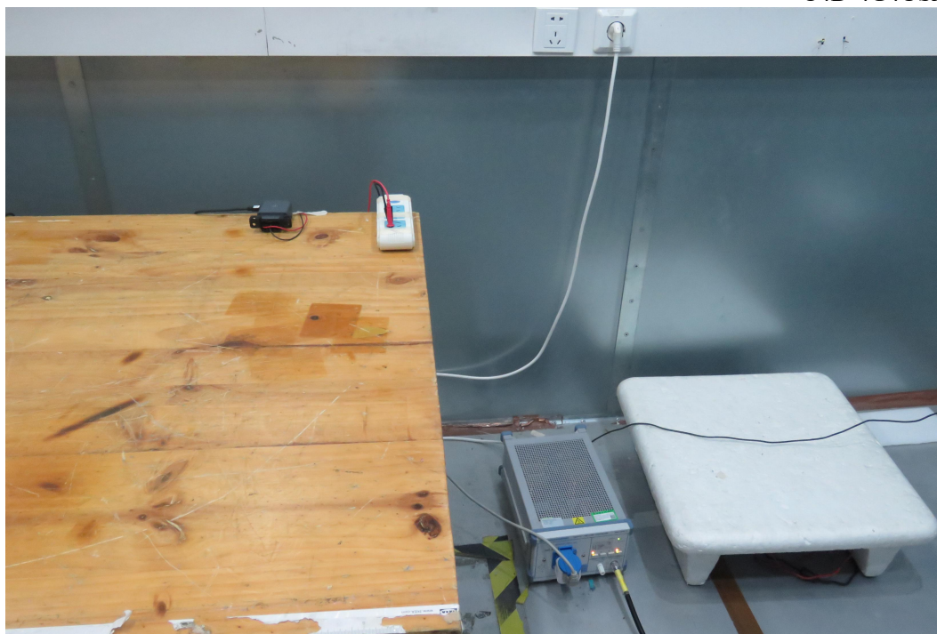
Picture 3 Conducted Emission Test Setup
