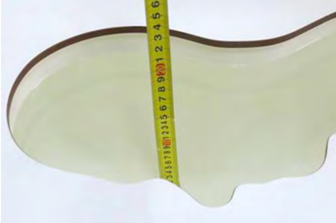
Picture 3: liquid depth in the head Phantom
