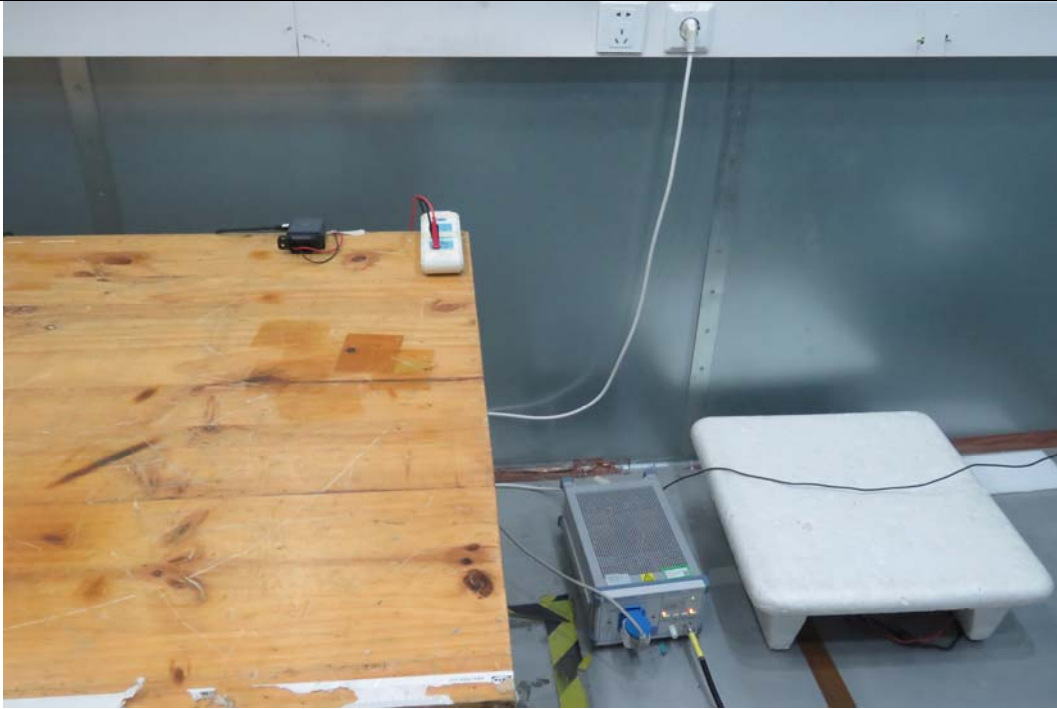
Picture 3 Conducted Emission Test Setup
