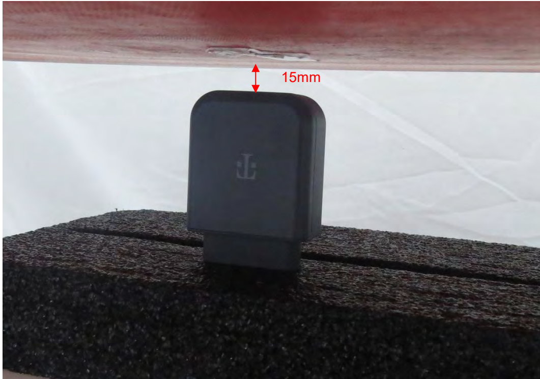
Picture 10: Bottom Side, the distance from handset to the bottom of the Phantom is 15mm
