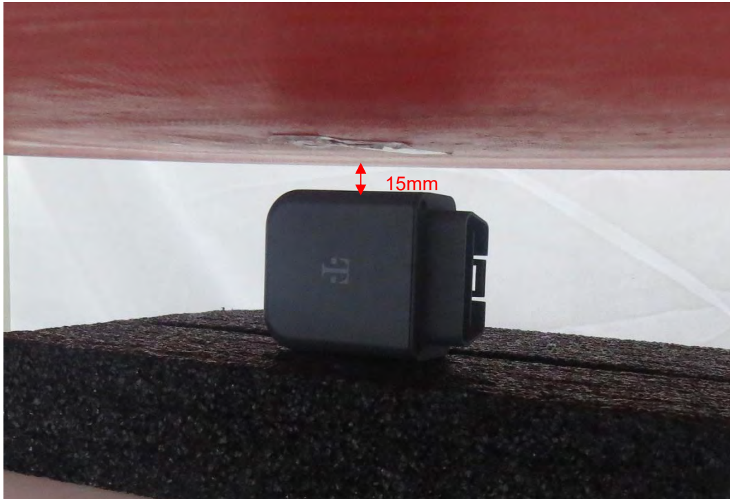
Picture 8: Left Side, the distance from handset to the bottom of the Phantom is 15mm
