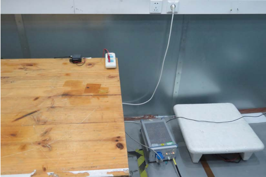
Picture 3 Conducted Emission Test Setup
