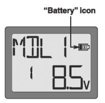
**Note**: If the transmitter ever reaches 8.9 Volts, land as soon as safely possible. A more reasonable margin of safety would be to quit flying for the day (or recharge the batteries) when the transmitter battery reaches 9.4 Volts.
