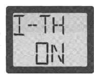
3. Push "SELECT" key to select the desired curve point. Point 1 is shown initially which is throttle stick's all the way downward (slow) position. Point 5 is throttle stick's all the way upward (hi) position.
