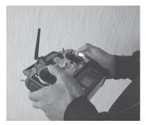
will give the best results. Please adjust the transmitter antenna to the way you hold the transmitter.
