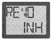
Press DATE "+" key, This will cause the flashing "INH" display to change to a flashing "ON" display. Now the "REVO" function is on.
