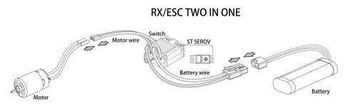
WARNING: MAKE SURE MATCH THE POLARITY (+/-) AS SHOWN ON THE BATTERIES. INCORRECT INSTALLATION OF BATTERIES WILL HARM THE FS-2REE! !!
