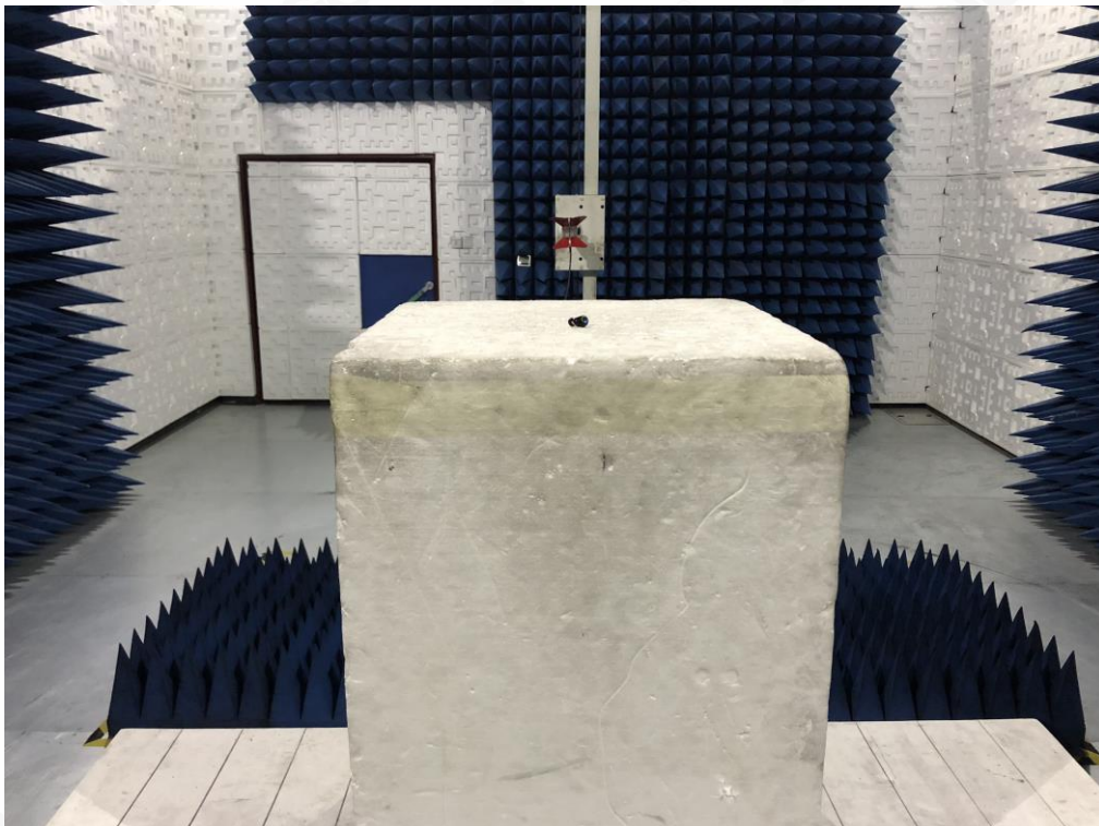
RADIATED EMISSION TEST SETUP ABOVE 1GHZ
