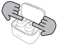
The earphones are in charging and the red light is on, press the left and right metal buttons for 3 times, the blue light flashes for 3 times, the reset is successful.
