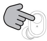
Press the left earphone for 0.5 seconds and make a beep, turn the volume up a notch.
