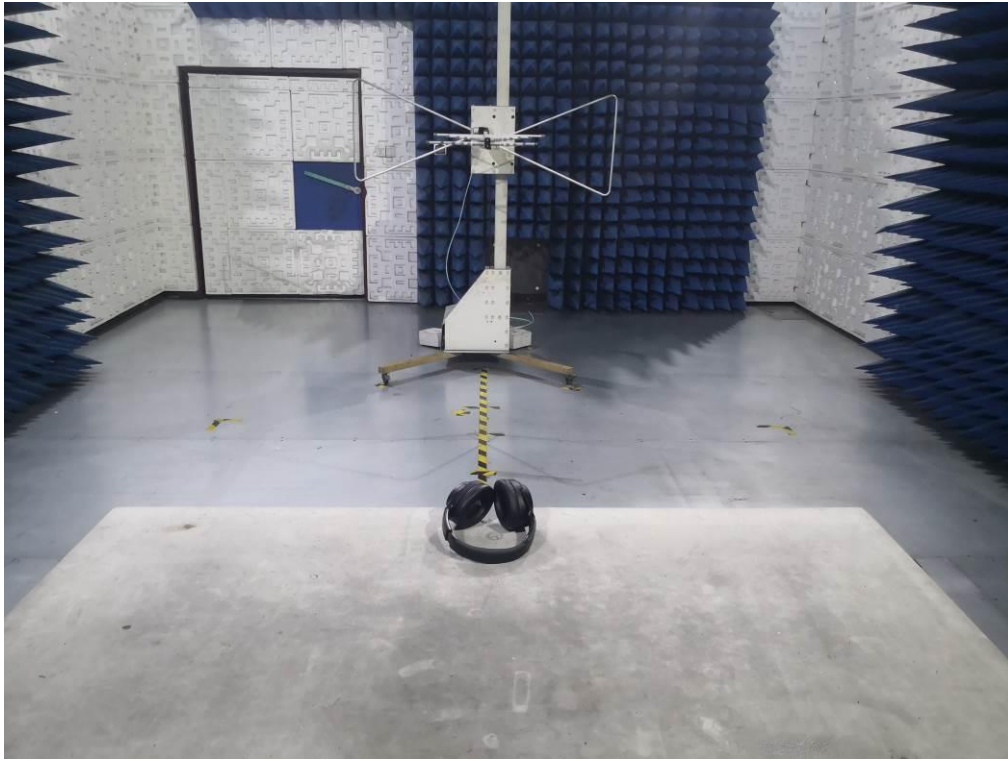
RADIATED EMISSION TEST SETUP ABOVE 1GHz
