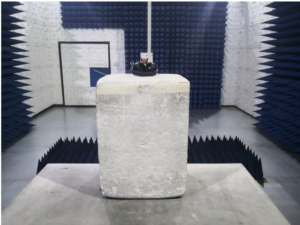
RADIATED EMISSION TEST SETUP ABOVE 1GHz
