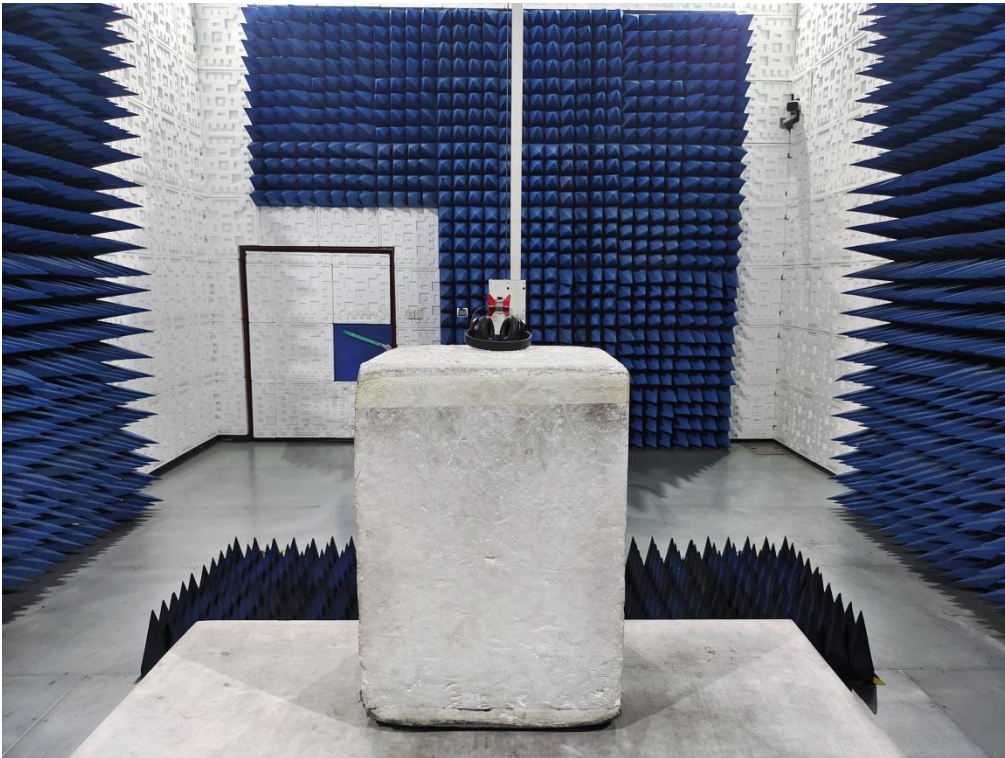
RADIATED EMISSION TEST SETUP ABOVE 1GHz
