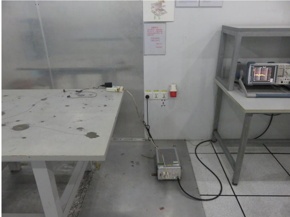
Photo of Conducted Emission Test
