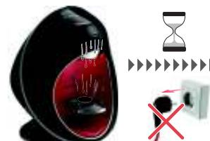
3 Coffee mix is pressed out of top of capsule holder. **Do not unplug the machine.** Wait until pressing process is finished. This is the case if you hear no noise coming from the machine.
