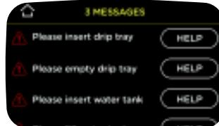
Tapping on **HELP** will display an instruction for resolving the defect.
