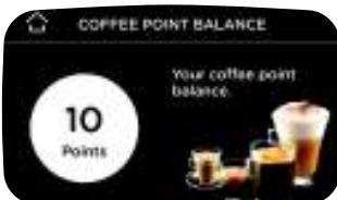
i Machine shows number of coffee points after each capsule preparation or by placing RFID card near RFID logo on the machine. Each beverage preparation deducts one coffee point.
