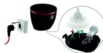
8 Unplug power plug! Take out the injector tool and the 2nd injector from the bottom of the capsule bin.
