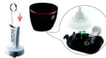
14 Insert cleaning needle into blocked injector to unclog it. If not possible, prepare a descaling solution with one part descaler solution to 0.5 litres of drinking water. Submerge blocked injector in the descaling solution.
