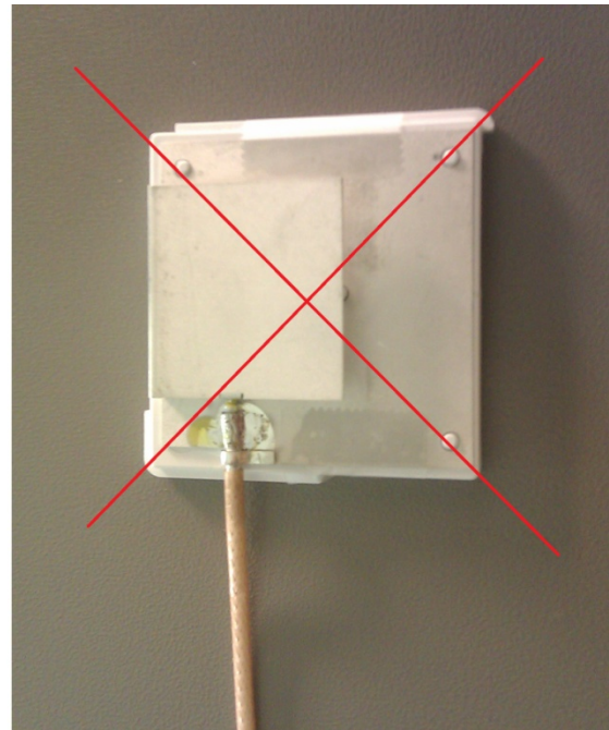
Figure 6: INCORRECT PIFA Mounting
