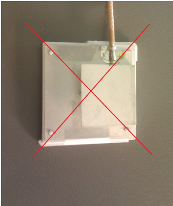
Figure 6: INCORRECT PIFA Mounting
