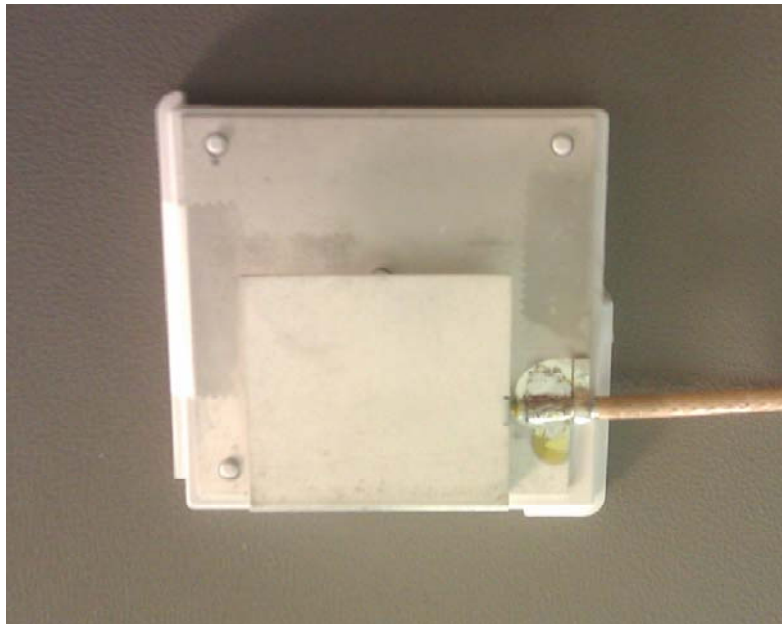
Figure 5: PIFA mounted near the bottom of an appliance (Cover removed). Open end pointed up.
