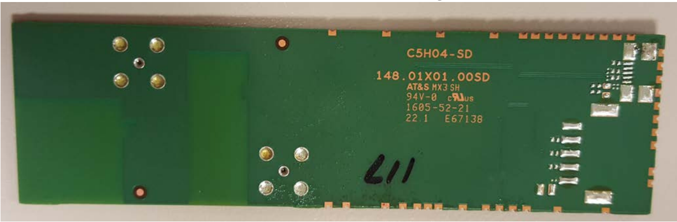
Circuit Board with On-board Antenna Configuration – Side 2
