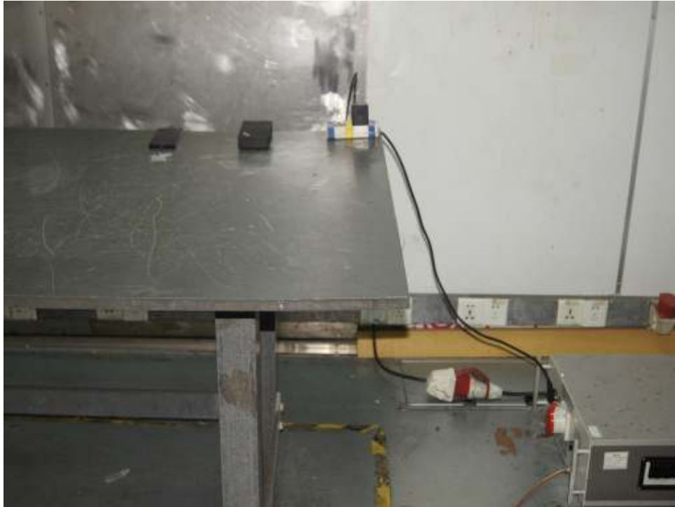
Photograph 7: Set-up for Conducted emissions
