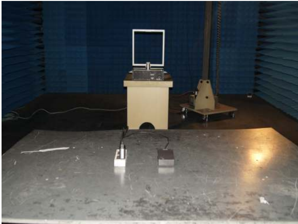
Photograph 2: Set-up for Spurious Emissions (30MHz-1GHz)
