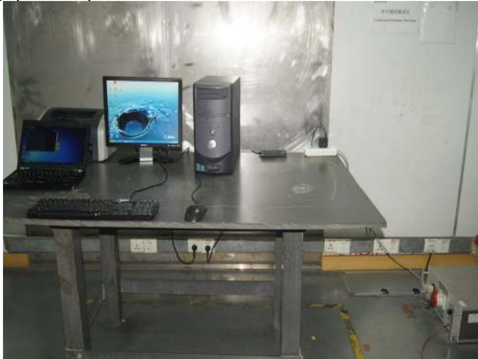
Photograph 2: Set-up for Radiated Emissions below 1GHz
