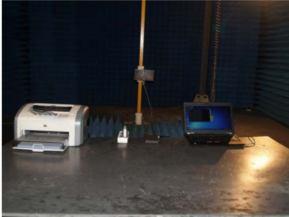
Photograph 3: Set-up for Radiated Emissions above 1GHz
