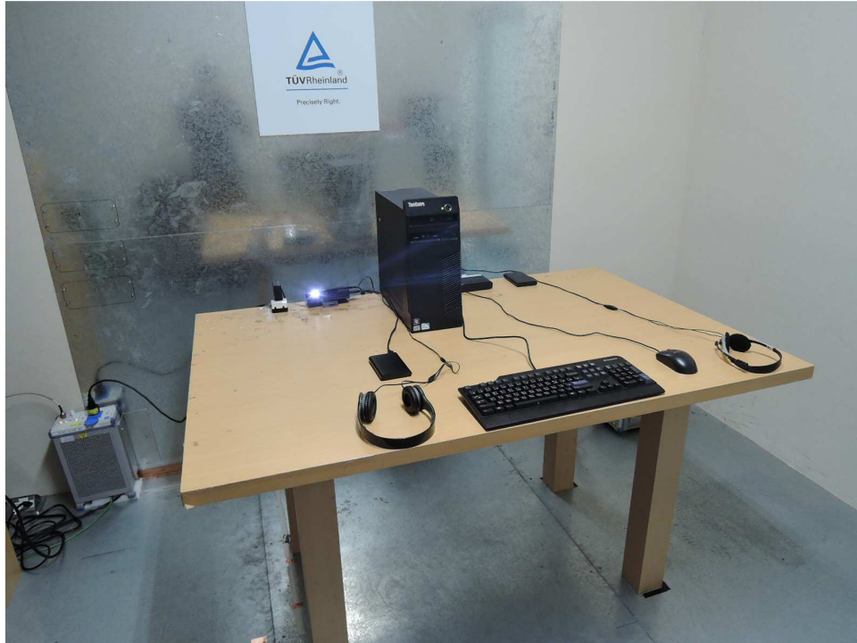
Photograph 6: Set-up for for Mains Conducted testing Front
