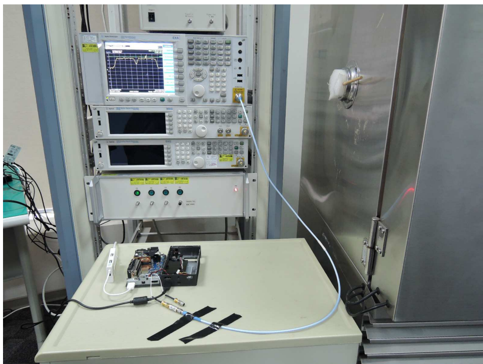
Photograph 4: Set-up for Conducted testing
