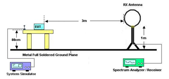
For radiated emissions from 30MHz to 1GHz
