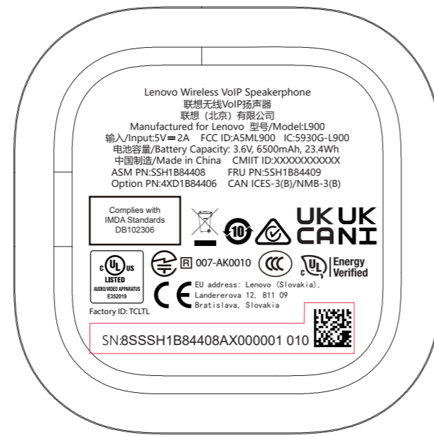
Label locates on the back of the device
