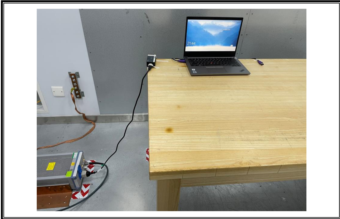
POWERLINE CONDUCTED EMISSIONS MEASUREMENT SETUP
