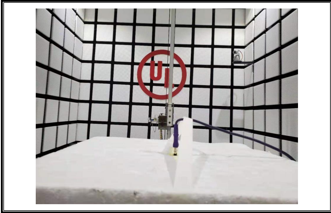
POWERLINE CONDUCTED EMISSIONS MEASUREMENT SETUP
