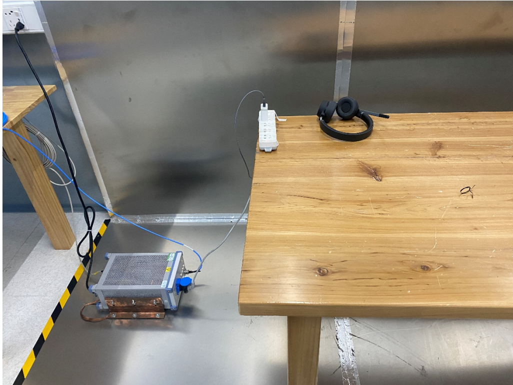
Photograph 3: Set-up for Conducted Emission on AC Mains
