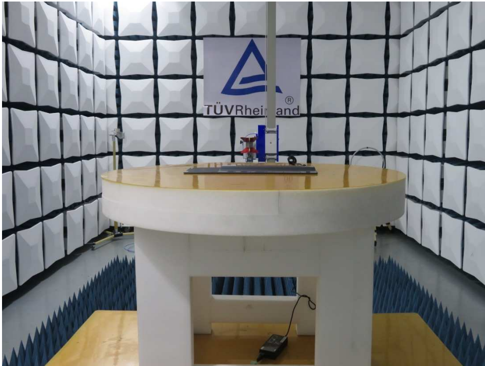
Photograph 3: Set-up photo for Radiated Spurious Emission, above 1GHz
