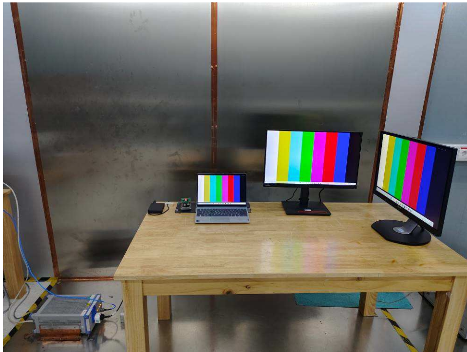
Photograph 1: Set-up for Conducted Emission on AC Mains
