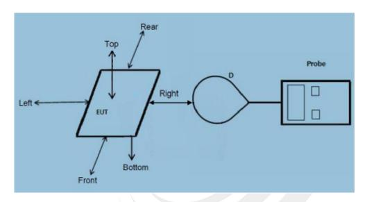
Remark: The E300 probe antenna diameter is 11.5cm.
