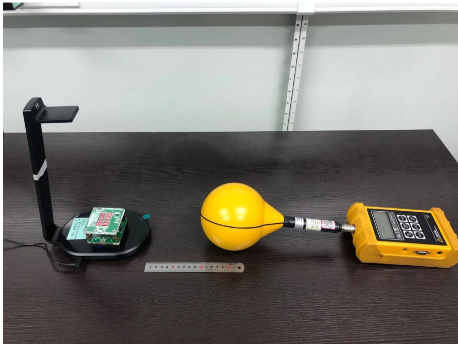
Photograph 4: Set-up photo for RF Exposure
