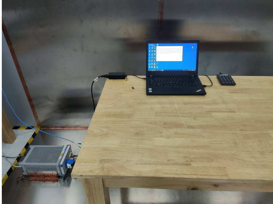
Photograph 3: Set-up for Conducted Emission on AC Mains
