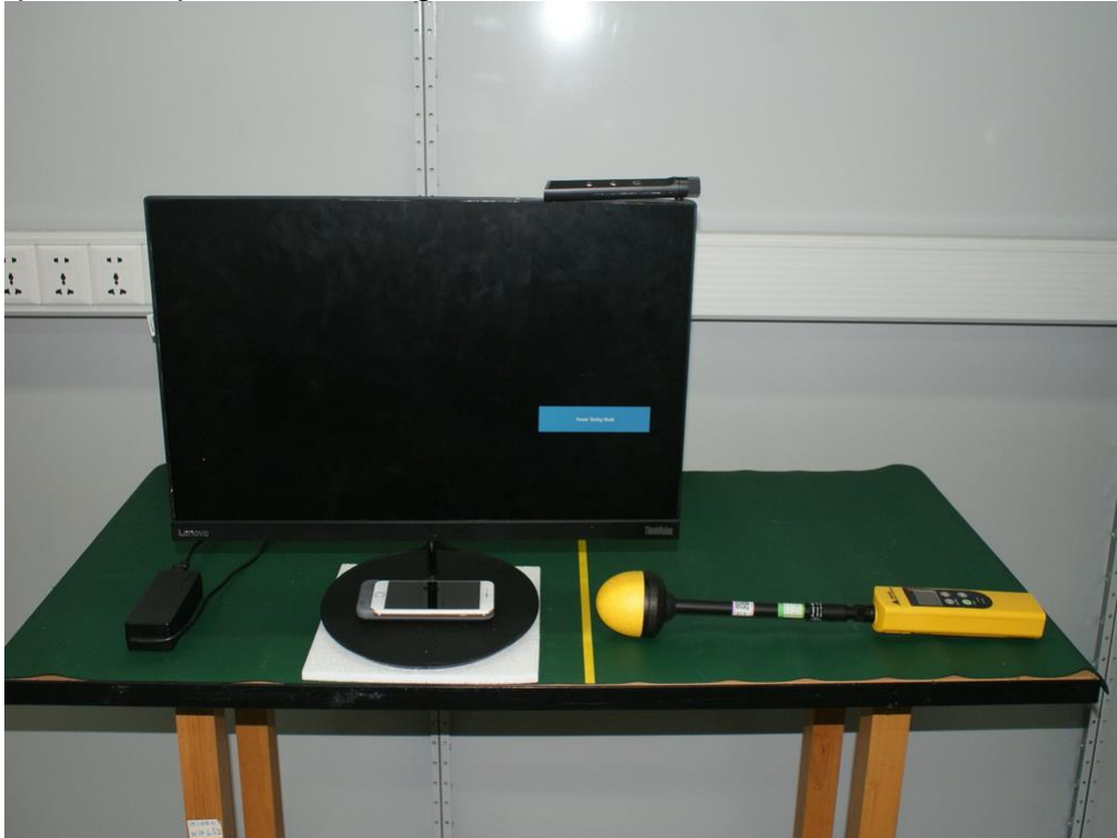
Photograph 1: Setup for Electromagnetic Fields
