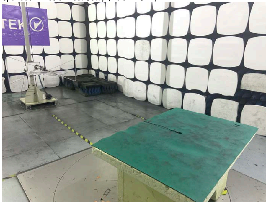
Spurious Emission Test Setup (Below 1GHz)
