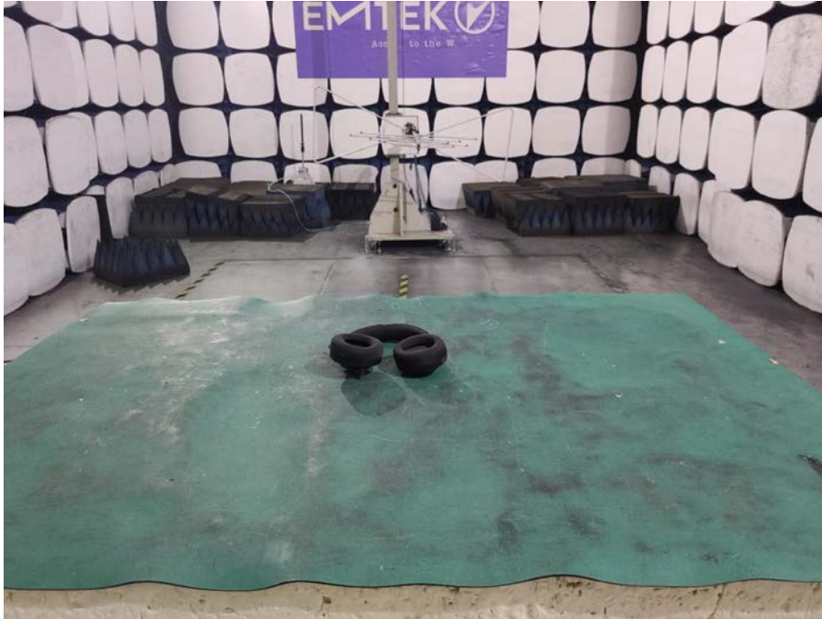
Spurious Emission Test Setup (Below 1GHz)
