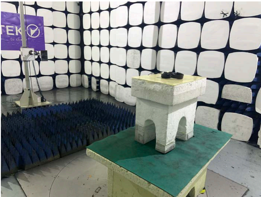
Spurious Emission Test Setup (Above 1GHz)
