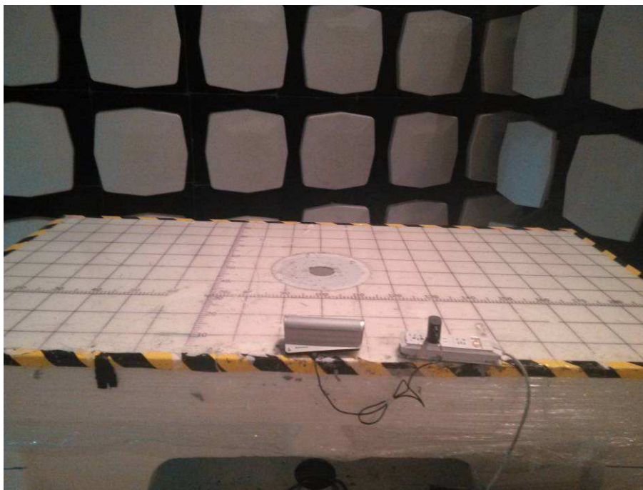
Test Setup Photo –Radiated Emission
