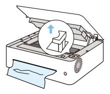
3 Pull the jammed paper carefully out of the paper exit.
