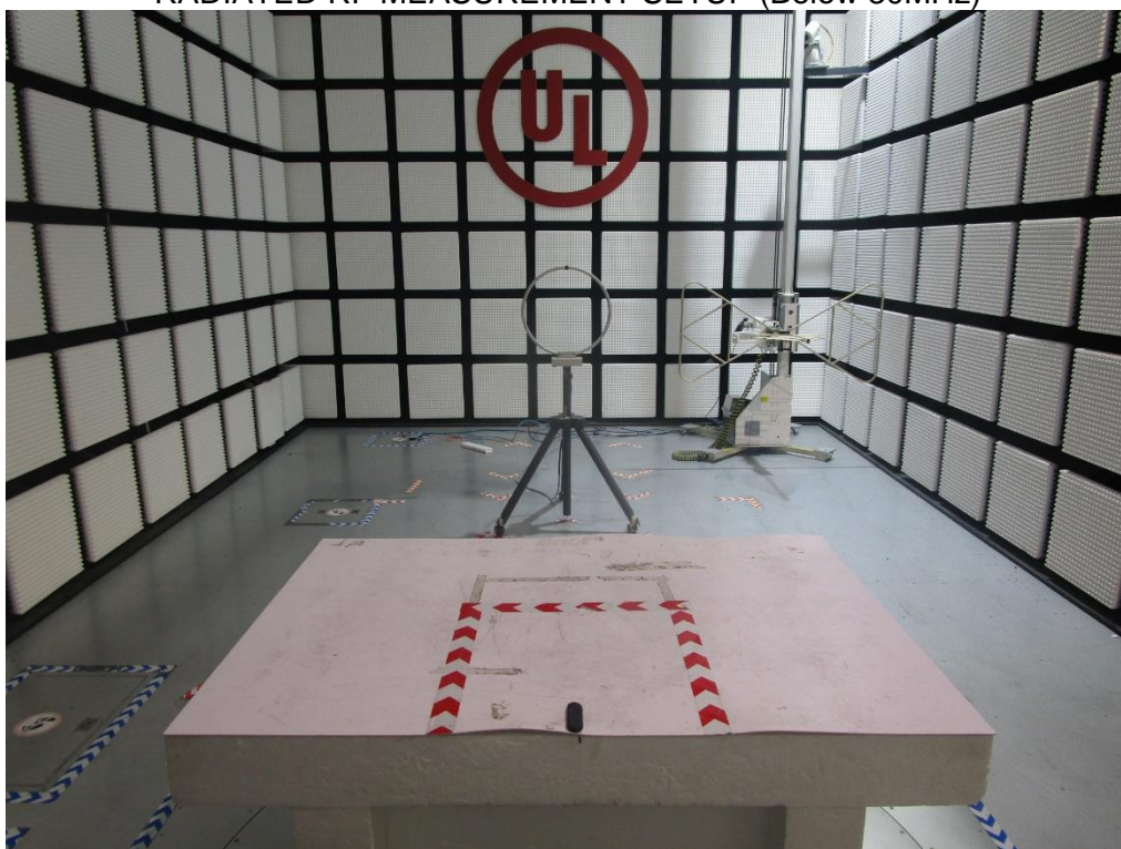
RADIATED RF MEASUREMENT SETUP (Below 30MHz)
