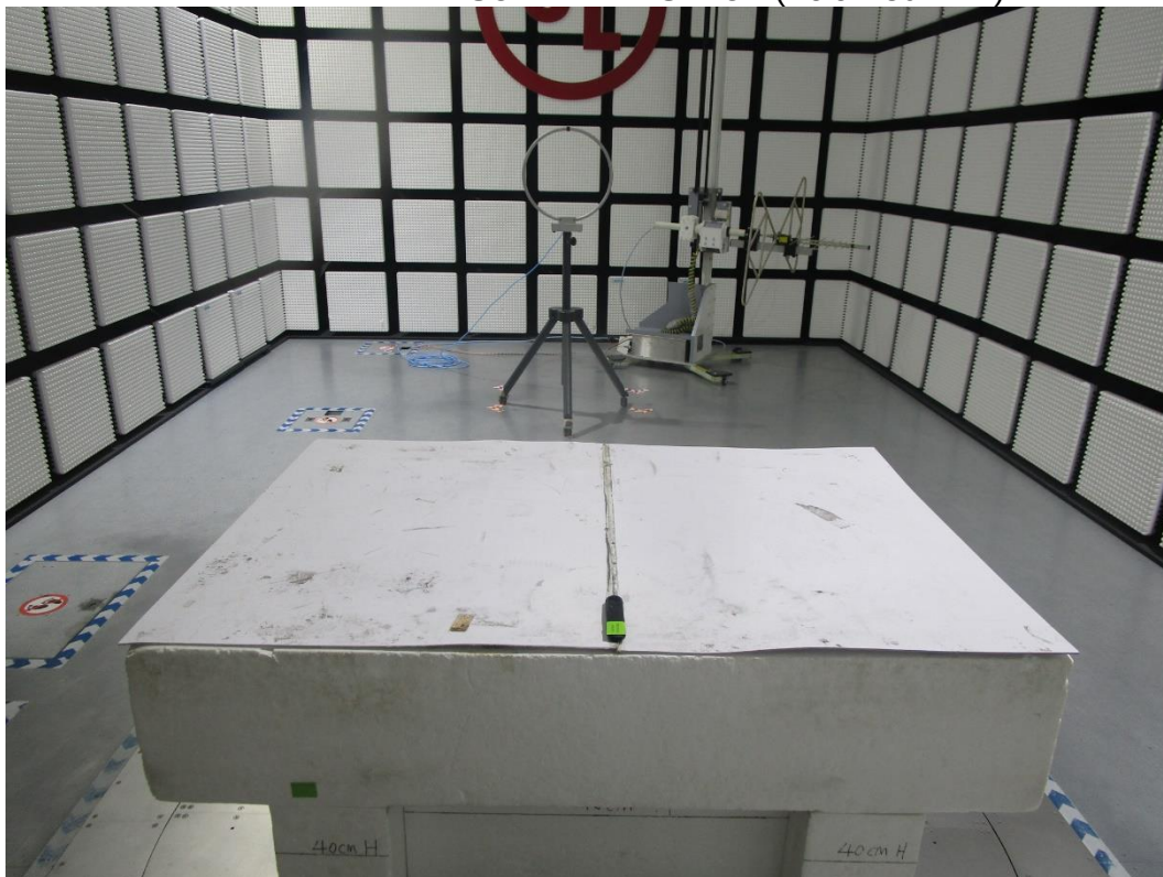
RADIATED RF MEASUREMENT SETUP (Below 30 MHz)
