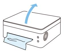
2 Pull the release lever upwards.
