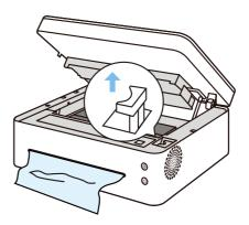
3 Pull the jammed paper carefully out of the paper exit.
